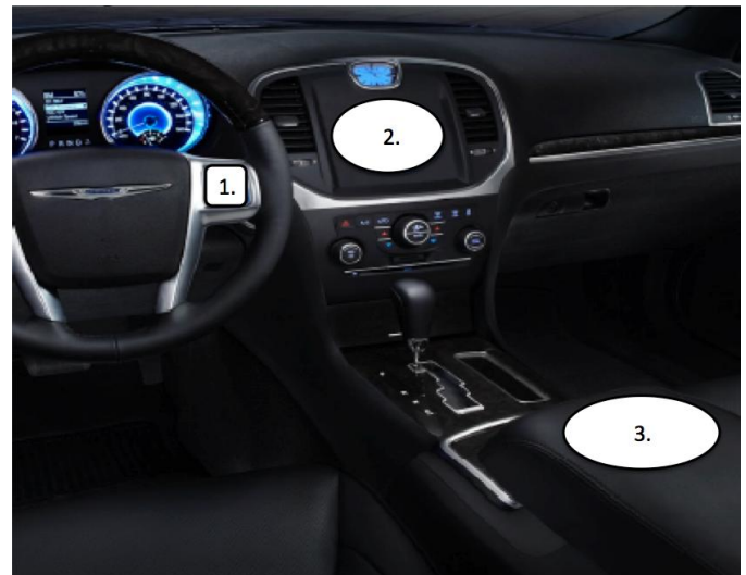
Figure 1. The three white areas indicate the steering wheel (1), center stack (2) and armrest (3) test locations.
